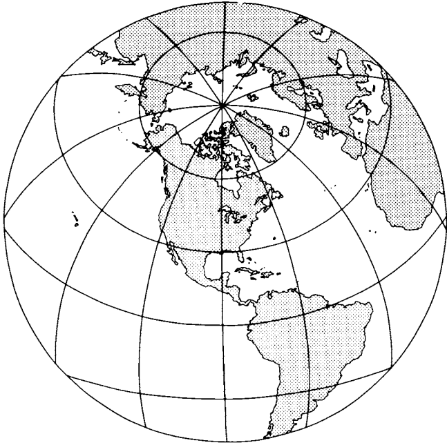
FIGURE 2.8. Oblique azimuthal equidistant projection centered on Chicago, Illinois, just east of the meridian at 90^\circ W.
